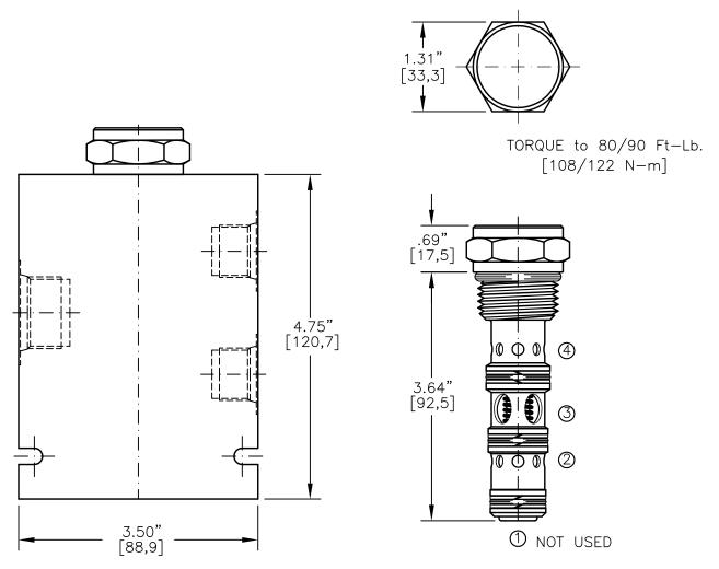
PORT #3 (INLET) IS ONE SIZE LARGER THAN PORTS #2 & #4 (OUTLETS). FOR ALUMINUM OR STEEL VALVE HOUSING CONFIGURATIONS SEE PAGE 0-043.2
